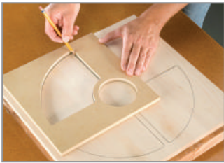
Trace the templates onto the bowl blank.
