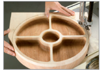
Bandsaw the exterior to final shape.
