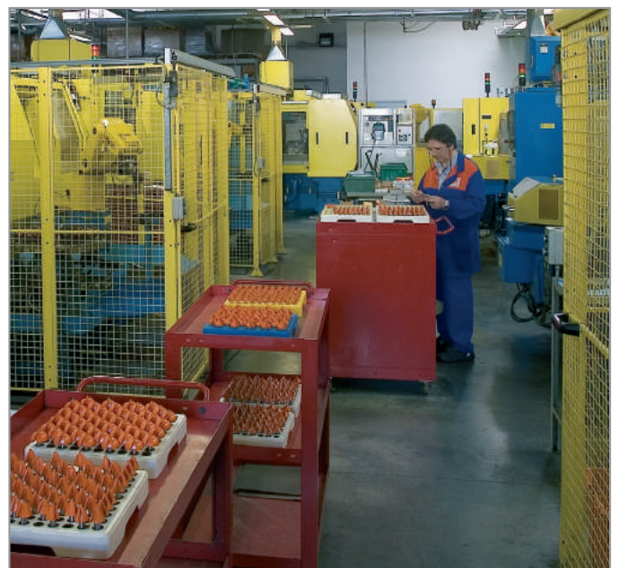
Loading the automated multi-axis CNC sharpening machines.
