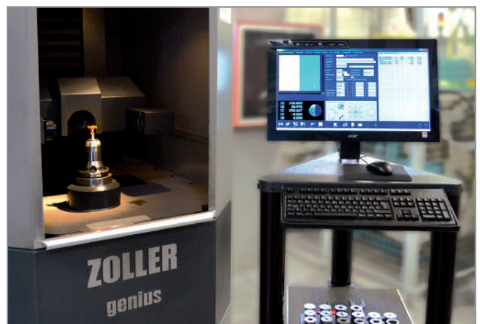
CMT's fully automatic measuring system.
